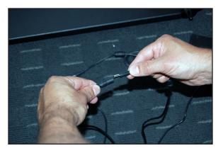
4. At the back of the display connect the two cords from the bottom of the lightbox into the power supply cords. Then plug into your electric source and turn on.
