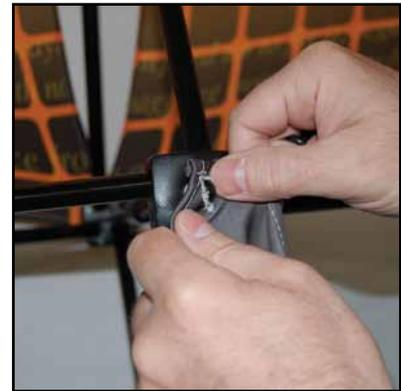
6. Start at the top left or right hub and push button hole in skin corner over the hub node. Attach the remaining 3 corners the same way.
