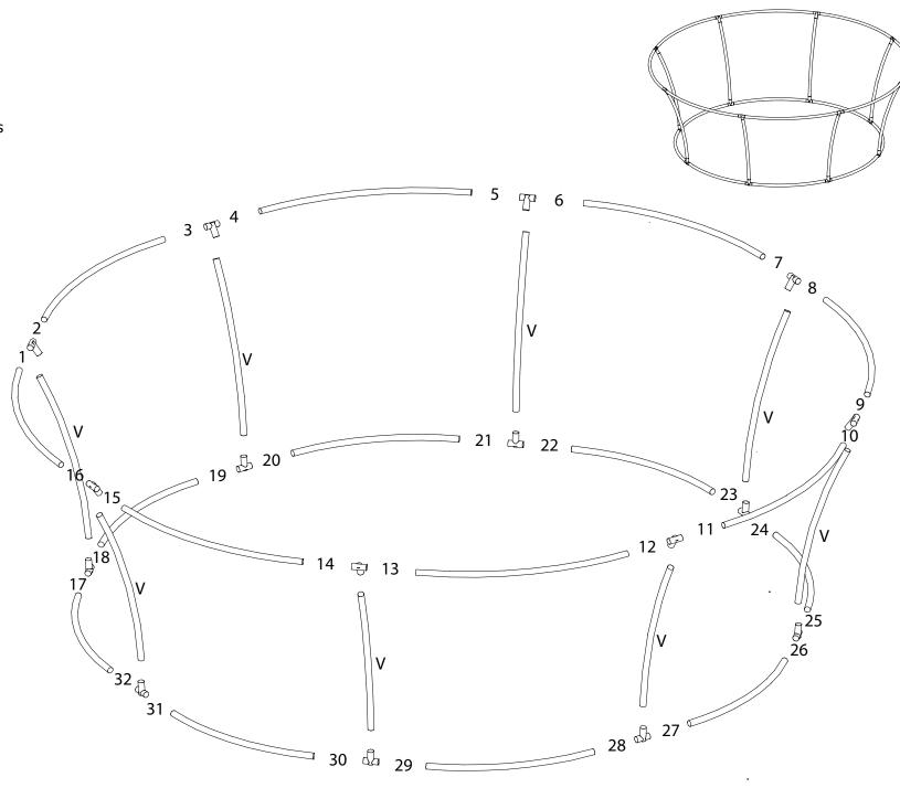
1) Connect all pieces together. 2) Connect lower section and upper section together using (8) Vertical Supports.
