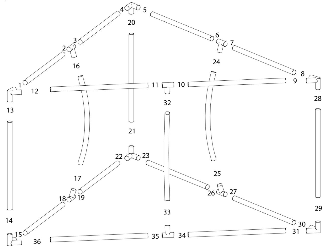
Assemble Aero Frame together in numerical order as shown.
