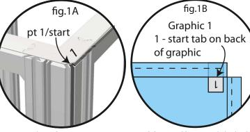
Step 1 - Identify start point on top of frame (fig. 1A, label-1) and graphic top left corner with start tab (fig. 1B, shown in blue).
