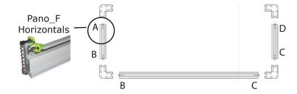
Step 2 - Place assembled vertical posts down onto corner connector on horizontal section. Do one wall or section at a time. Tighten D screws on vertical posts.
